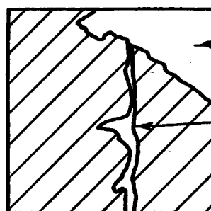
FIGURE 24. ELECTRON MICROGRAPH OF WELD METAL B SHOWING APPEARANCE OF CRACK
