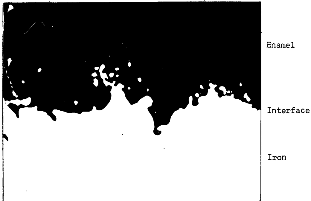
Figure 1.- Photomicrograph (X1,000, unetched) of metallographic section of porcelain-enamel ground coat containing 0.8 percent cobalt oxide applied to sandblasted enameling iron, showing rough interface between enamel and iron. This specimen had excellent adherence.
