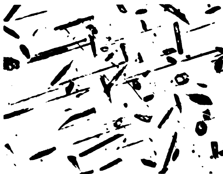
FIG. 4 5% COARSE SPECIMEN. MAGNIFICATION 600 X. 2000 CYCLES AT .001 STRAIN. DUPLEX MICRO-CRACKS RELATED TO DUPLEX SLIP.
