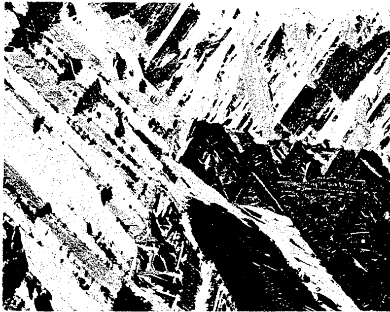
FIGURE 71. UNALLOYED PROCESS A TITANIUM WATER QUENCHED FROM 1700 F
