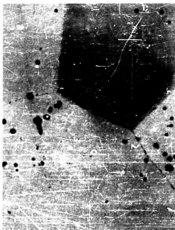
FIGURE 52 — MICROSTRUCTURE OF Mo-AL-Nb ALLOY, HEAT B179 0.16% ALUMINUM, 0.5% NIOBIUM, BALANCE MOLYBDENUM, CAST IN ARGON ELECTROPOLISHED, ETCHED IN SODIUM HYDROXIDE + POTASSIUM FERRICYANIDE SOLUTION
