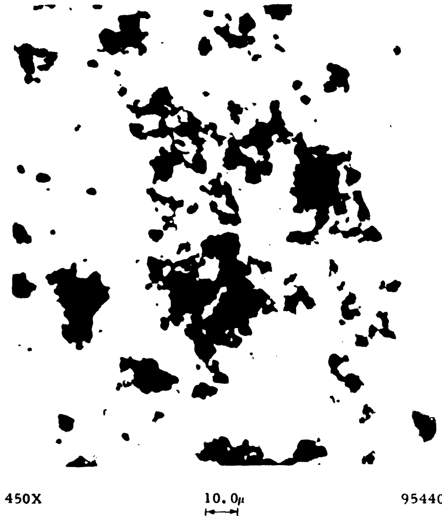
FIGURE 10-29. PHOTOMICROGRAPH OF POWDER PARTICLES PRODUCED BY POWDER-CLOUD GENERATOR
