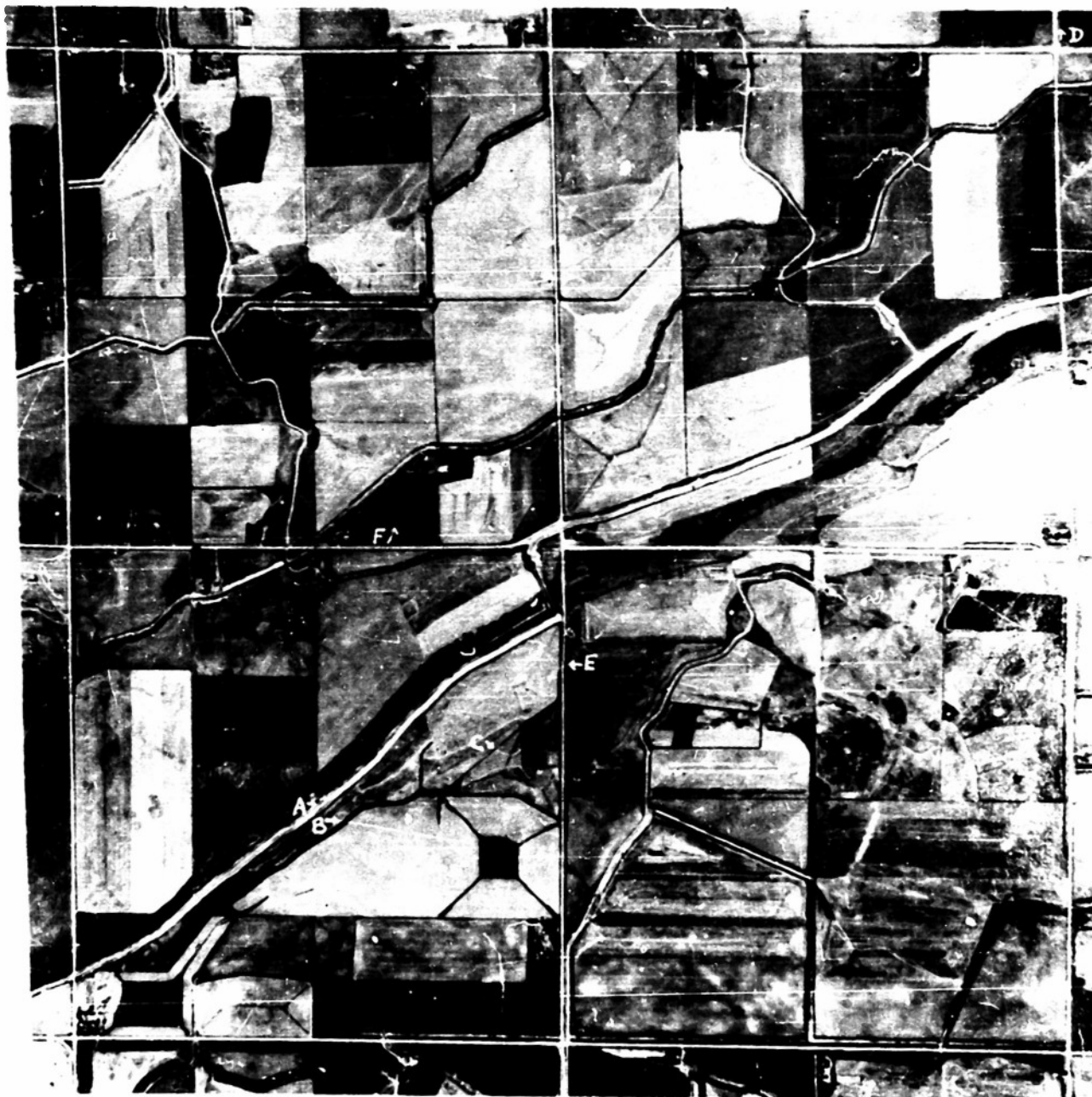
Photo 2. Aerial view of distribution features. This shows principal distribution features of Greenfields Irrigation District. (A) Greenfields Main Canal (B) Lateral (C) Sub-lateral (D) Head Ditch (E) Border Ditch, and (F) Field Ditches. Scale 1:20,000. (USDA, 1951, Photo ZS-10H-6).
