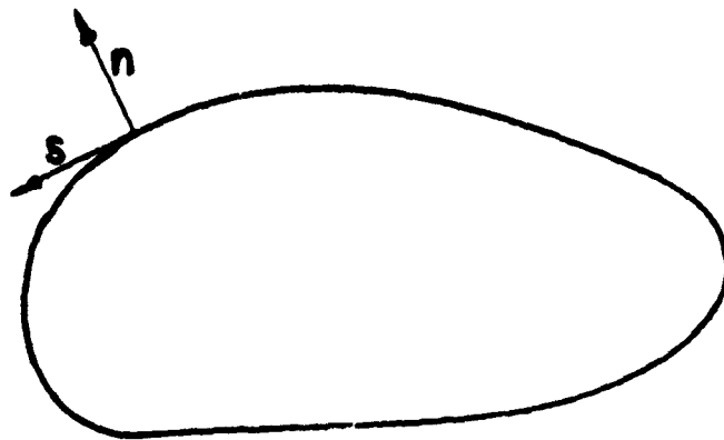
(a) Curvilinear plate showing normal and tangent at point on boundary.
