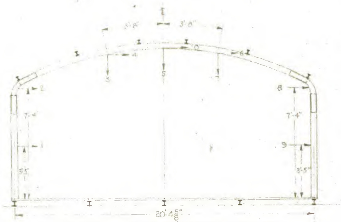
FIGURE 9. LOCATION OF DEFLECTION GAGES ON RIGID FRAME
