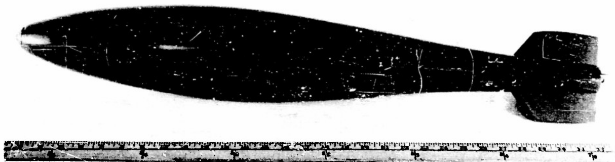
Figure 3. Quarter-Scale Balsa Model
