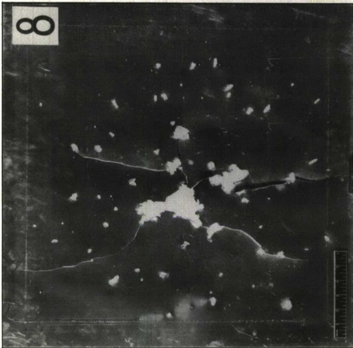
b Manufactured by British Aluminium Co. Ltd. to Spec. D.T.D.687 (Analysis C2) - .064 in. Thickness (16 S.W.G.) "Burster" to Test Plate - 19 in.
