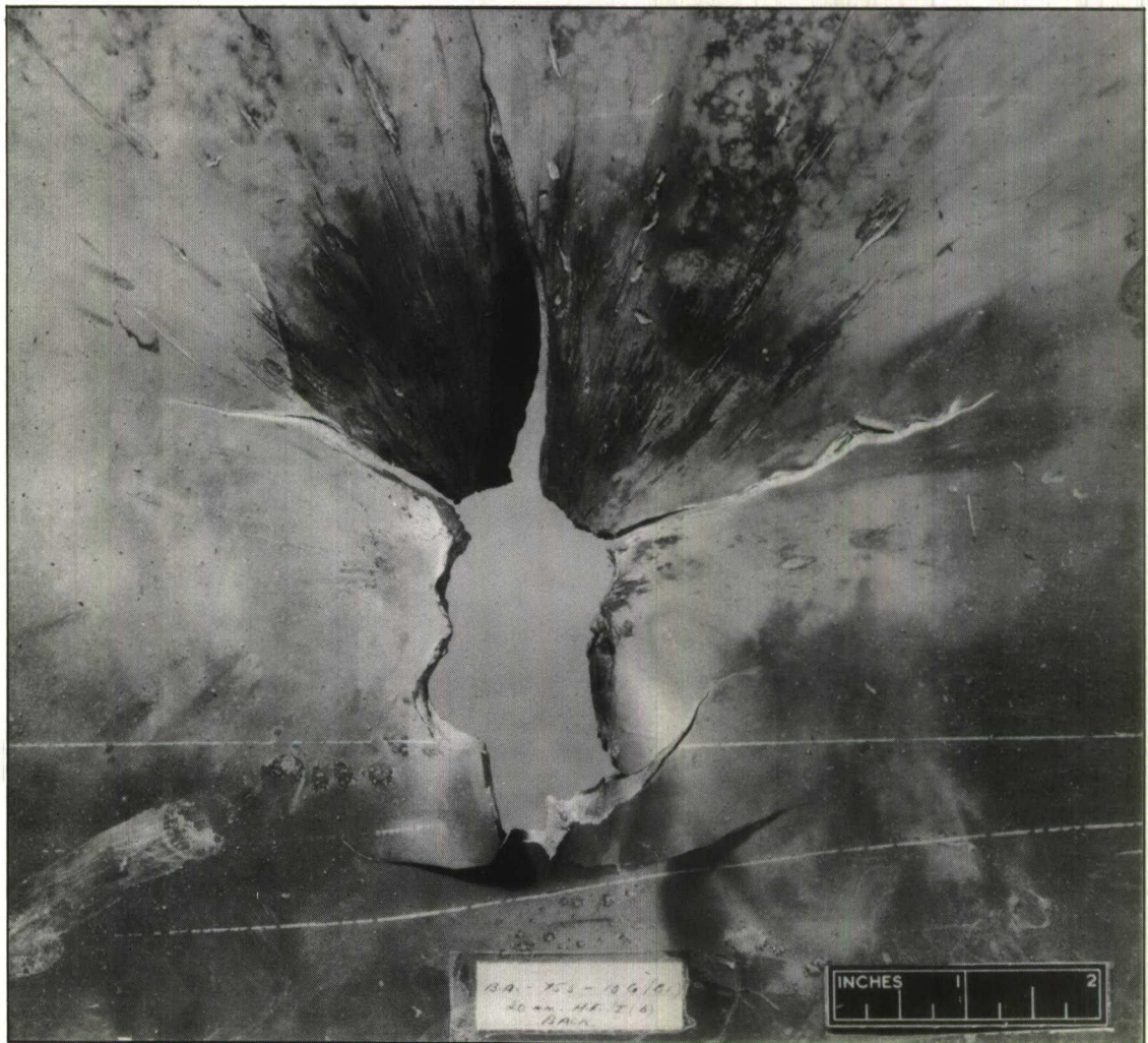
b. Firing 2. Exit Side. Detonation when Shell is in Plane of Plate.
