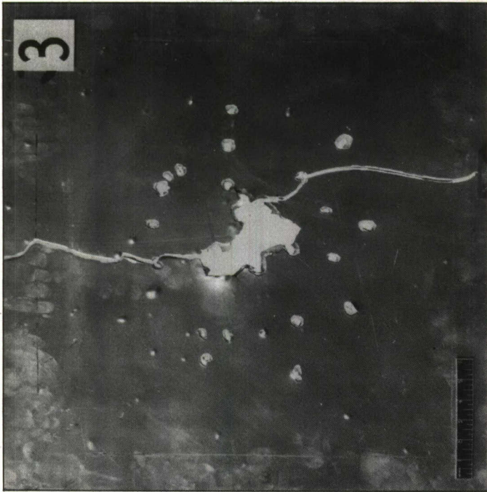
c Manufactured by Northern Aluminium Co. Ltd. to Spec. D.T.D.687 - 3/16 in. Thickness. "Burster" to Test Plate - 13 in.
