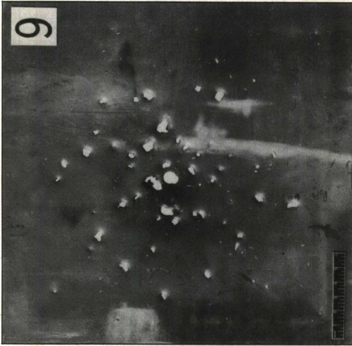
c Manufactured by British Aluminium Co. Ltd. to Spec. D.T.D.603 - .064 in. Thickness (16 S.W.G.) "Burster" to Test Plate - 19 in.
