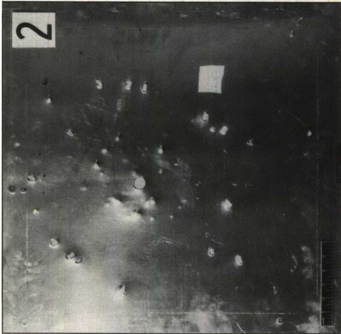
b Manufactured by British Aluminium Co. Ltd. to Spec. D.T.D.687 (Analysis A2) - 3/16 in. Thickness. "Burster" to Test Plate - 19 in.
