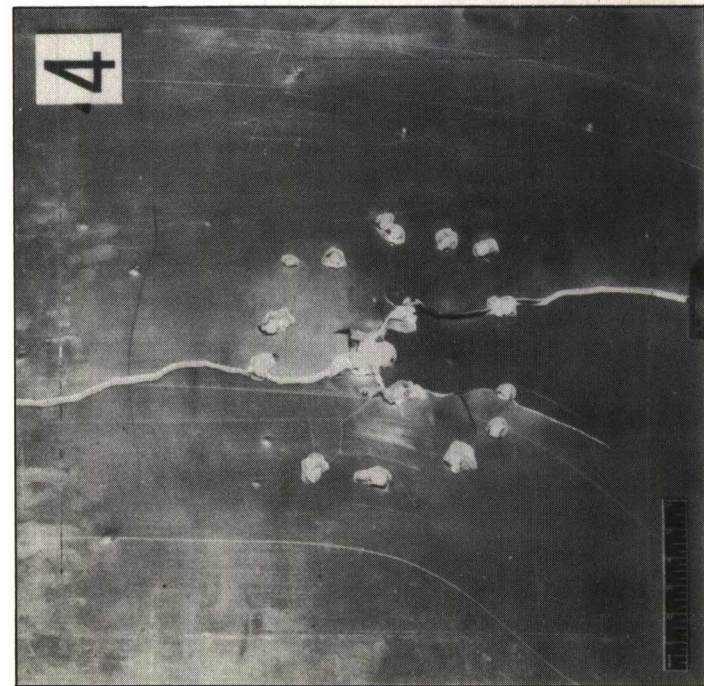
a Manufactured by Messrs. James Booth and Co. Ltd. to Spec. D.T.D.687 - 3/16 in. Thickness. "Burster" to Test Plate - 13 in.
