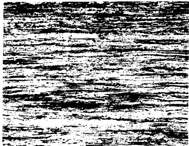
AS ROLLED INITIAL PASSES 1150-1240°C FINAL PASSES 925°C 85% REDUCTION 200 X
