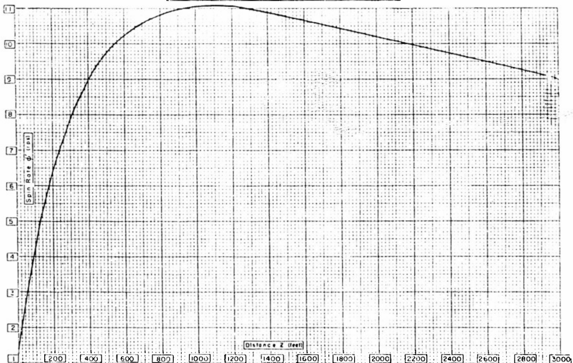
Fig. 4. Rolling Velocity Versus Distance From Gun. Calculated From Roll Equation For T119E11 Projectile.
