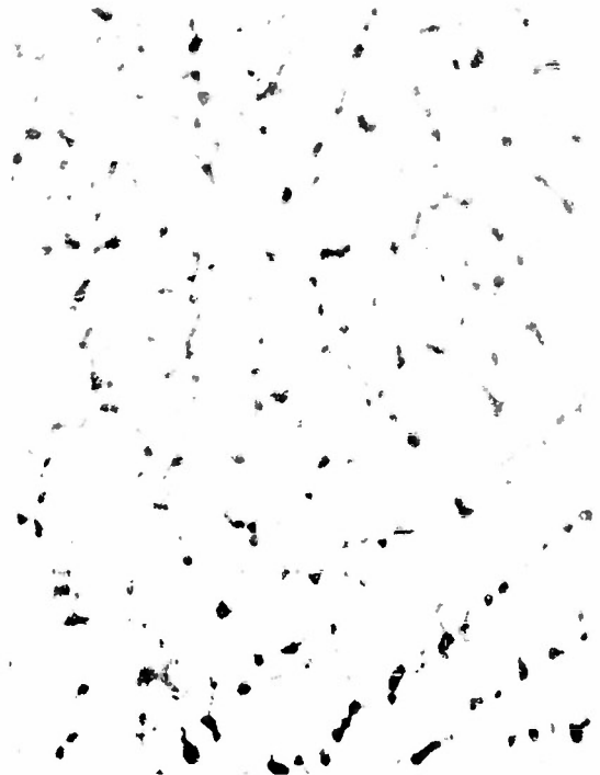
(B) ELECTROPOLISHED, ETCHED IN SODIUM HYDROXIDE + POTASSIUM FERRICYANIDE SOLUTION, X100 (M2470)
