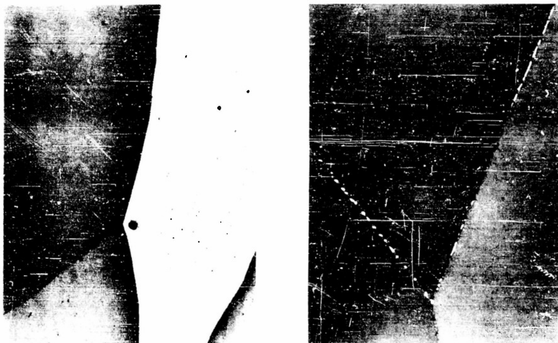
FIGURE 114 - MICROSTRUCTURE OF Mo-Co-Ti ALLOY, HEAT B208 0.06% Co, 0.70% Ti, 0.020% C, balance molybdenum, cast in vacuum Electropolished, etched in \text{NaOH} + \text{K}_3\text{Fe}(\text{CN})_6
