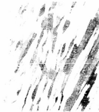
INGOT 1175 0.033% CARBON 1.46% VANADIUM CAST IN VACUUM (P970)
