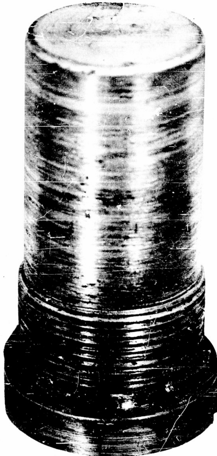
FIG. 4 EFFECTS OF GAS EROSION ON A NORMAL LEAD WASHER ASSEMBLED IN A MK 48 BASE FUZE CONFIDENTIAL
