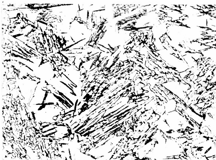
FIG. 14: STRUCTURE OF 4340 PRODUCED BY REACTION FOR 2 MINUTES AT 940°F FOLLOWED BY 50 SECONDS AT 660°F. NITAL ETCH. 800X.
