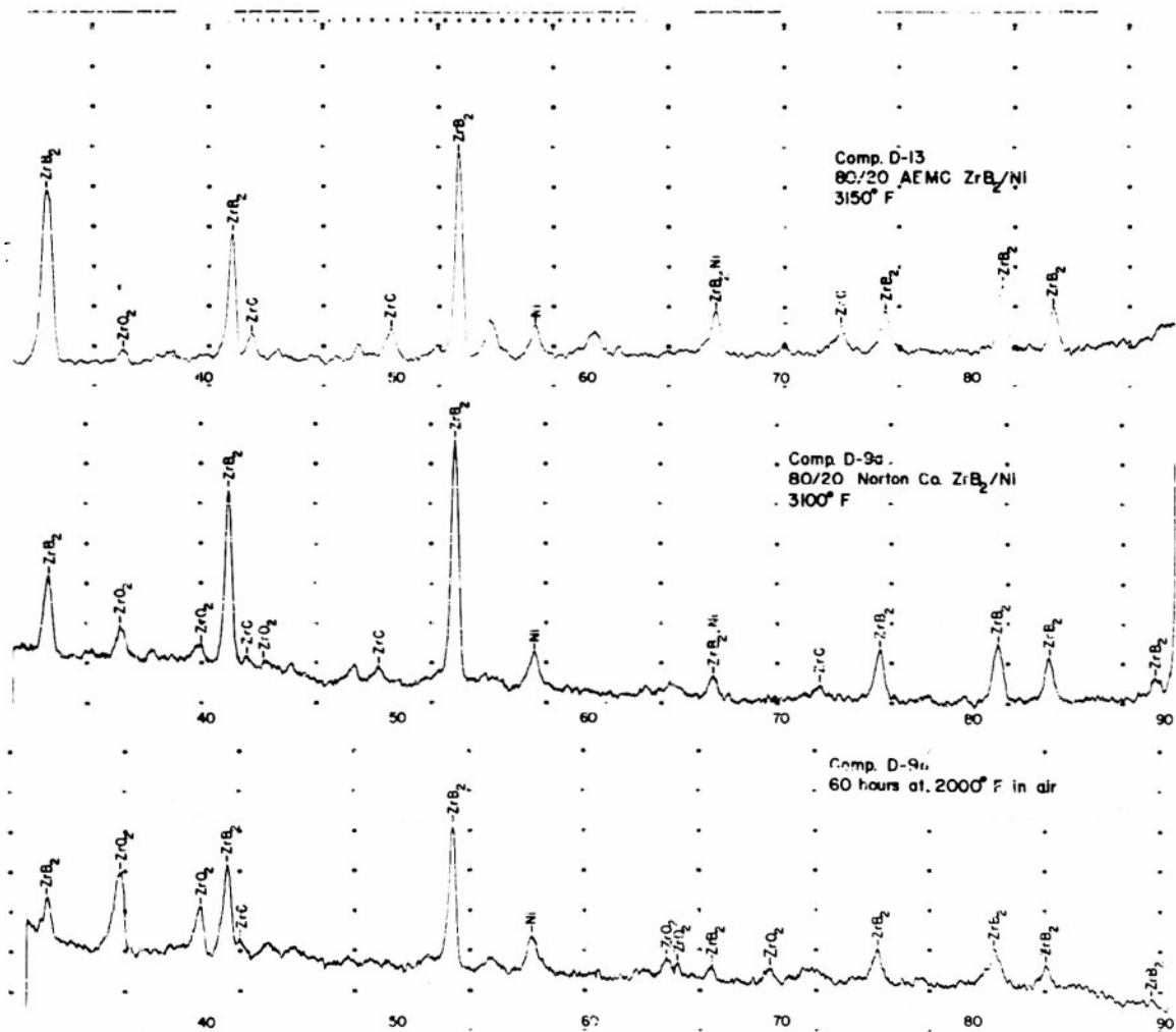
Figure 7. - X-ray Diffraction Patterns of Zirconium Diboride - Nickel Bodies
