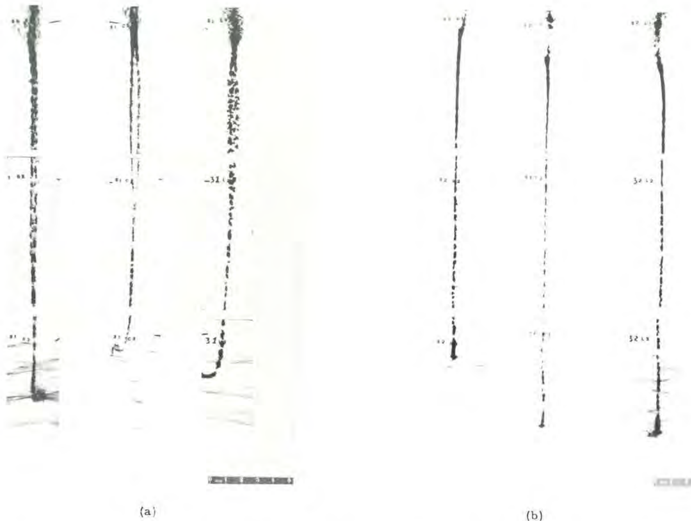
FIG. 2. Flash Radiographs of jets from 105mm fluted liners fired (a) statically, and (b) at optimum spin rate (45 r. p. s.). Comparison with similar photographs of jets from smooth liners shows clearly that the fluted liner fired at its optimum frequency produces a jet like that from a statically fired smooth cone, while the statically fired fluted liner produces a jet like that from a smooth liner fired at 45 r. p. s. The pictures show each jet at three different times and viewed from three different positions. The relative insensitivity to rotation of the front of the jet is evident in (a); the very rear of the jet is just newly formed and has not had time to spread at the time of the picture. Photographs by courtesy of L. Zernow, S. Kronman, and J. Simon, Ballistic Research Laboratories, Aberdeen Proving Ground.
