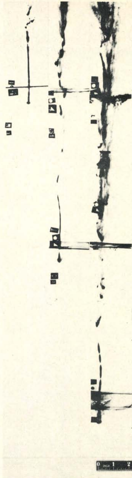
FIG. 1b. Radiograph of jet from 105mm copper liner after passing through five inches of glass protected by 1/2" steel and 1/4" rubber
