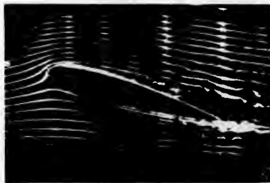
C. INCREASING ANGLE OF ATTACK
