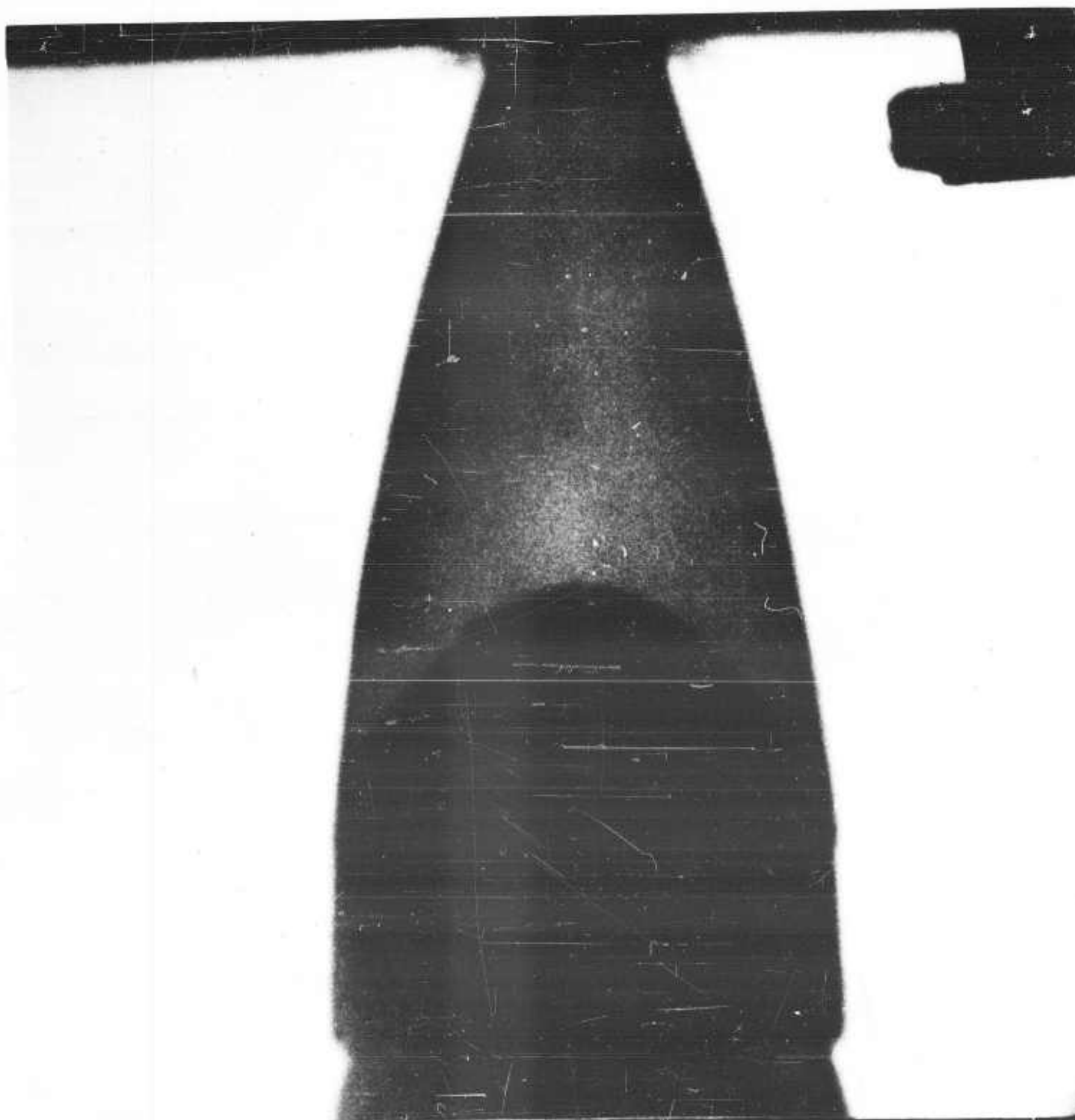
Flash x-radiogram of Butt Impact No. 4793 (APL). Dynamic deformation of a steel windshield.
