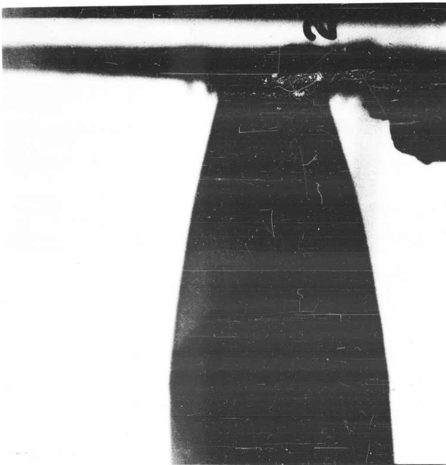
Flash x-radiogram of Butt Impact No. 4798 (APL). Dynamic deformation of a steel windshield.
