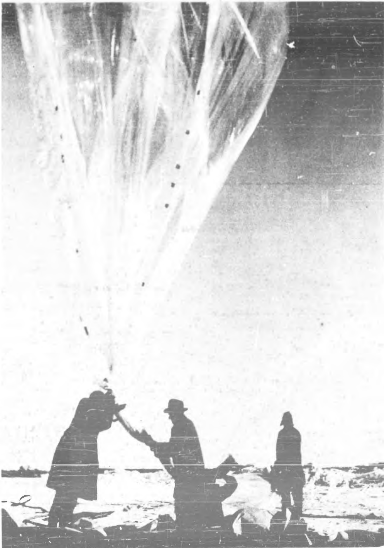
Figure III-3. After the weigh-off the temporary tie is removed and the balloon is allowed to become vertical, controlled gently in a hand-over-hand manner.
