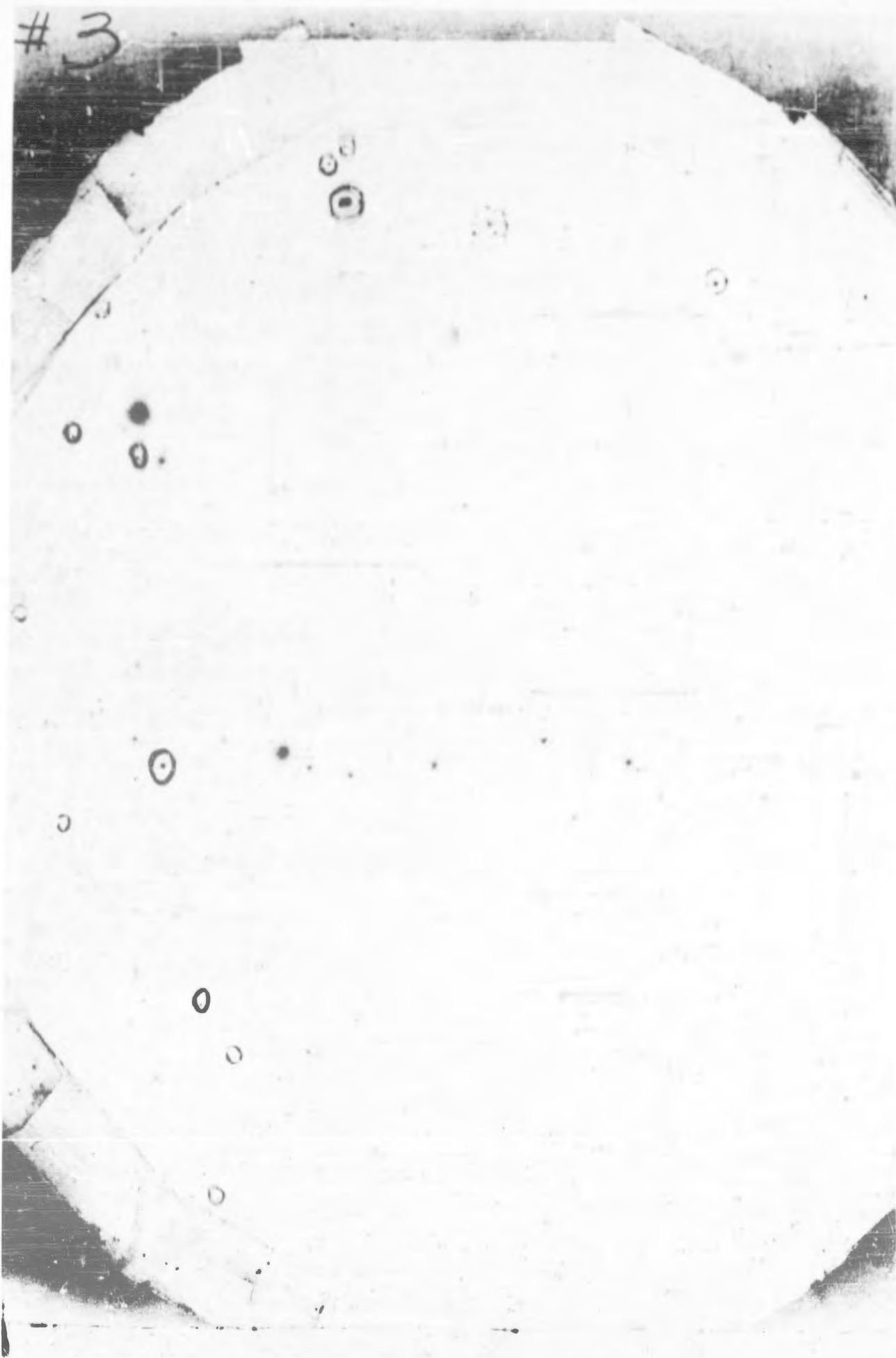
PLATE 10 -- Selenium Sulfide print of bad sample of "Mylar" showing pinholes (circled).
