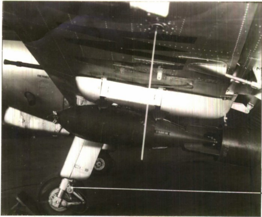
FIG.1. 250 LB. GP MK.4 BOMB ON 100/1000 LB. CARRIER UNIT WITH FAIRINGS FITTED.
