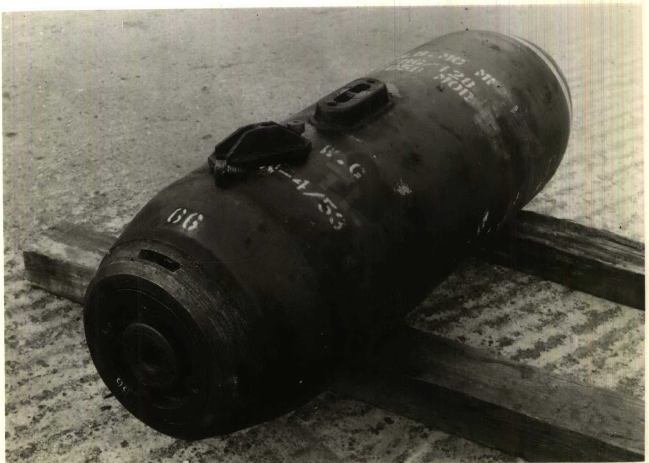
FIG.1b. 500 lb M.C. BOMB BODY Mk.18 SHOWING AFT END AND LIFTING PLATE
