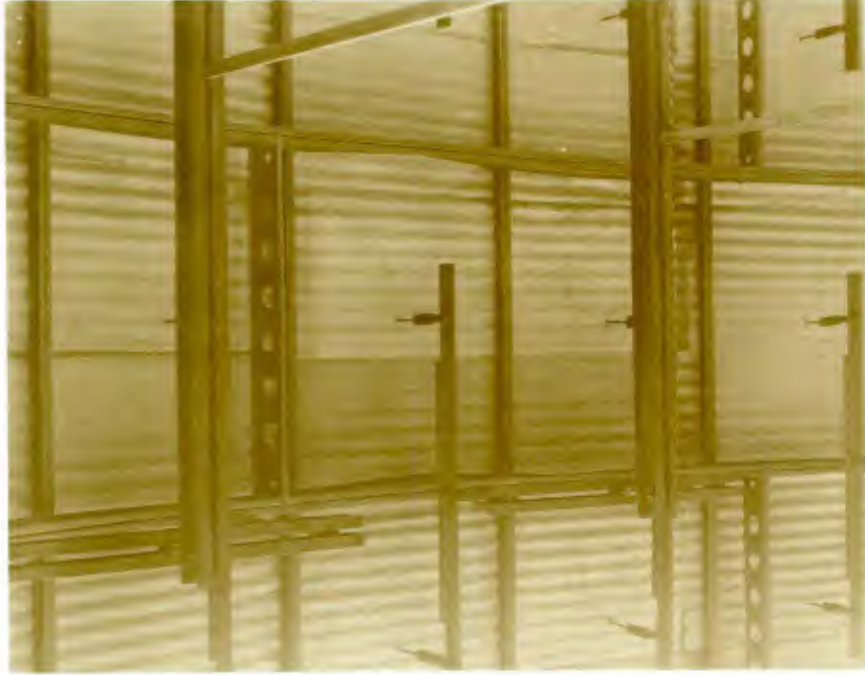
Figure 10. Ribs buckled at the top of the arch. The condition shown is at 185% of design load.
