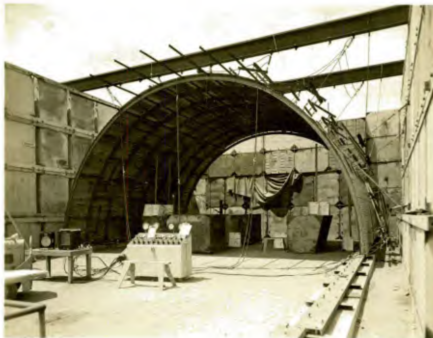
Figure 3. Test gear for applying a simulated wind load hydraulically using whiffletrees.
