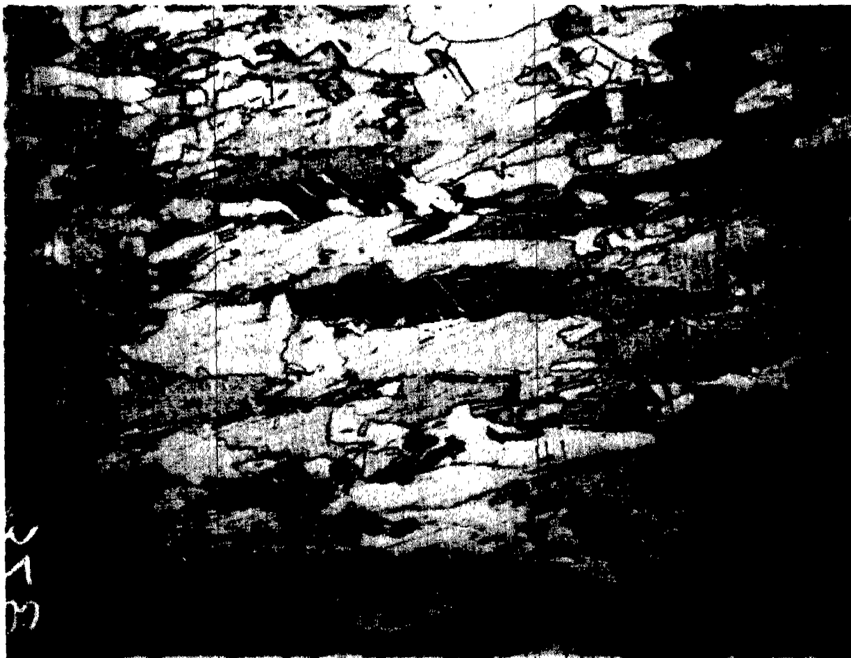
FIG. 41. Microstructure of recrystallized electrodeposited liners. (X100)
