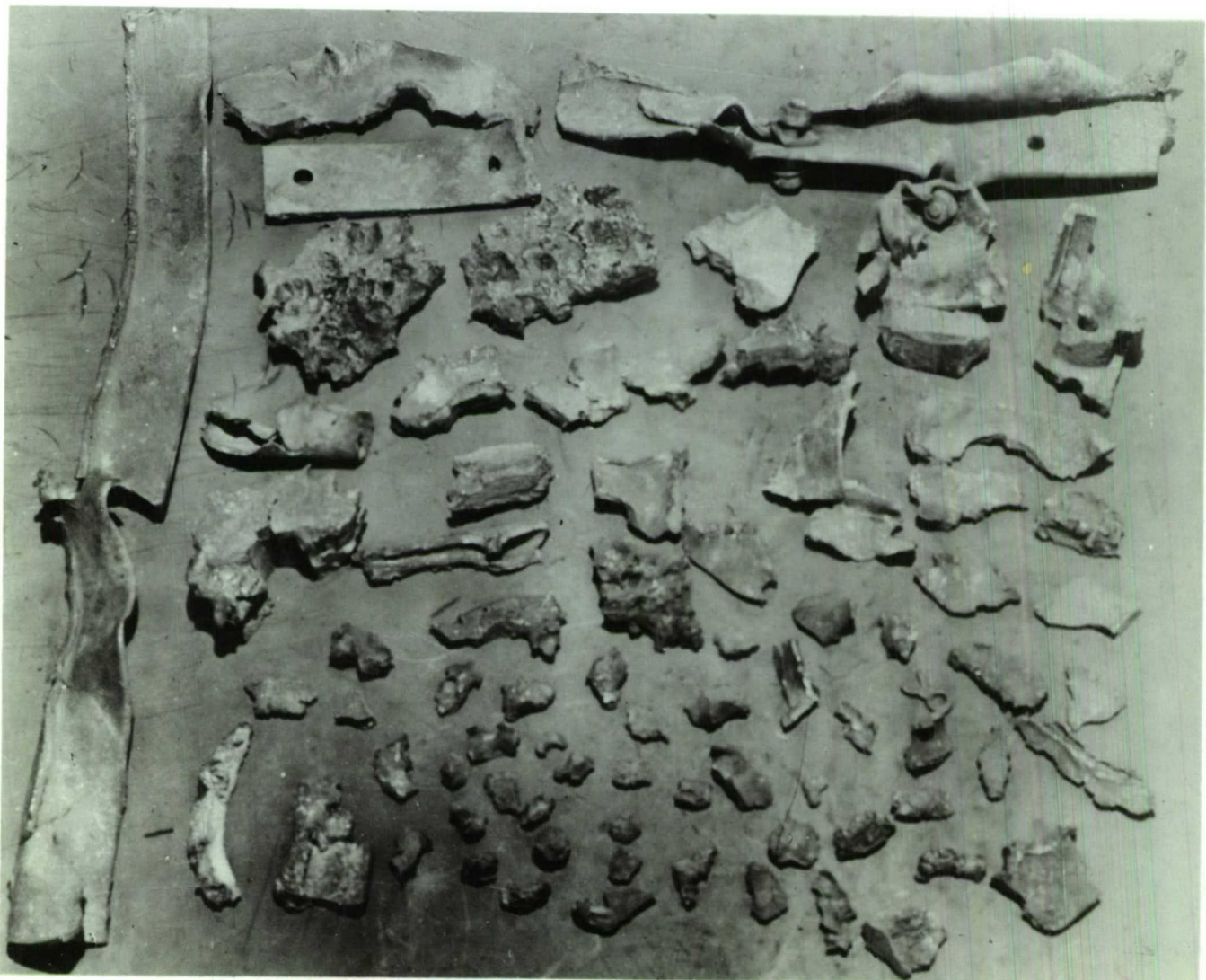
32. Fragments of apparatus recovered from crater after detonation of 1000 lb. bomb at Shoeburyness
