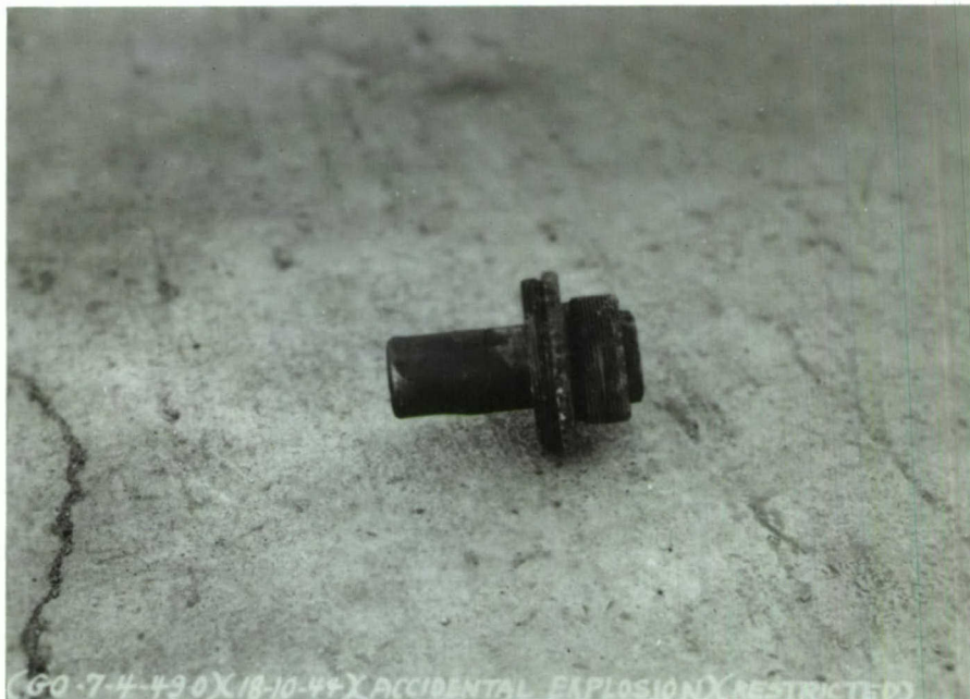
20. Exploder assembly after explosion of American bomb
