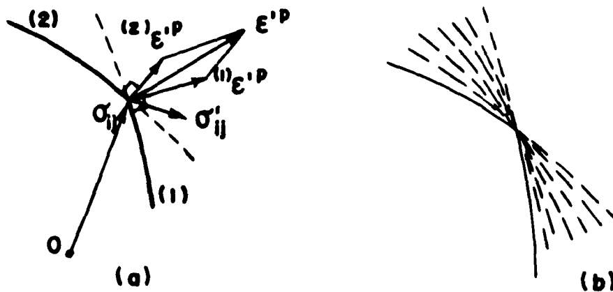
FIG. 4 A CORNER AS AN INTERSECTION OF TWO OR MORE LOADING SURFACES
