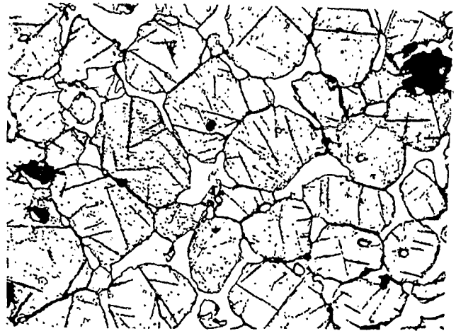
Fig. 8 Borolite IV 5/95 Heated in Air 1200°C 88 Hours
