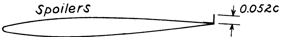
Figure 5.- Aileron and spoiler details. All dimensions in inches.
