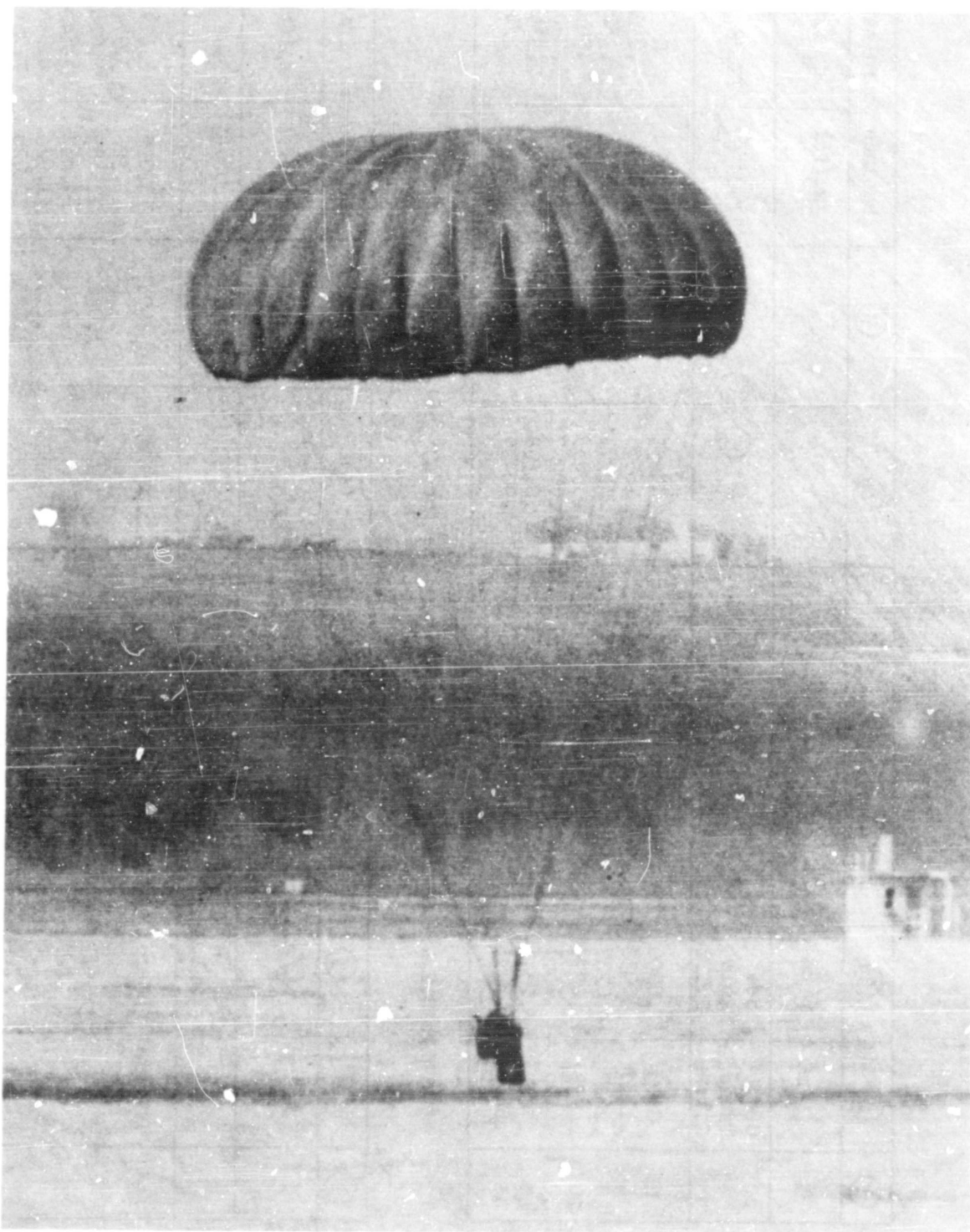
Figure 2.2.4 - Representative Photograph of a Fully Inflated Extended Skirt Canopy (T-10)
