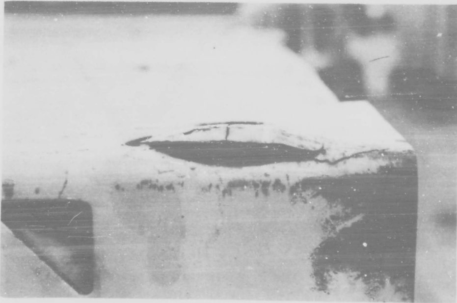
Figure 16. Corner strap failure on 3 x 12 ramp barge.
