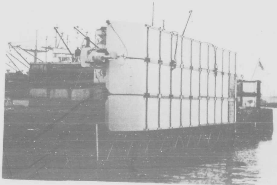
Figure 13. 3 x 12 ramp barge with O2D propulsion unit being launched from 5-ft 4-in. rail height.
