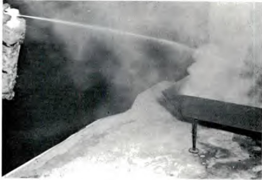
Figure 2. Pyrolyzed vapors resulting from extinguishing with Halon 1011 at -65 F clinging about fire area.
