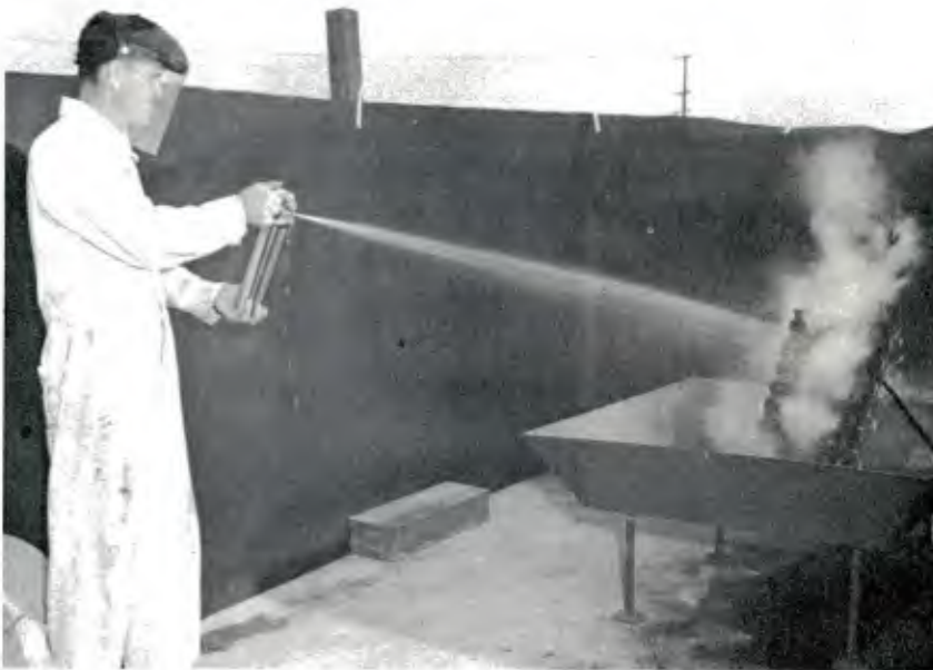
Figure 11. Extinguishing fire with zinc chloride at ambient temperature. Pyrolyzed vapors mostly steam.
