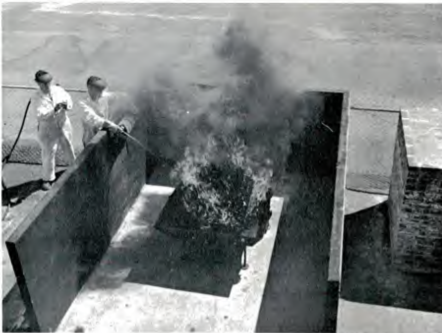
Figure 15. Deep-seated fire test with pyrolyzed vapors resulting from extinguishing with zinc chloride at -65 F. Vapors are not nearly as dense as those when Halon 1011 was used.
