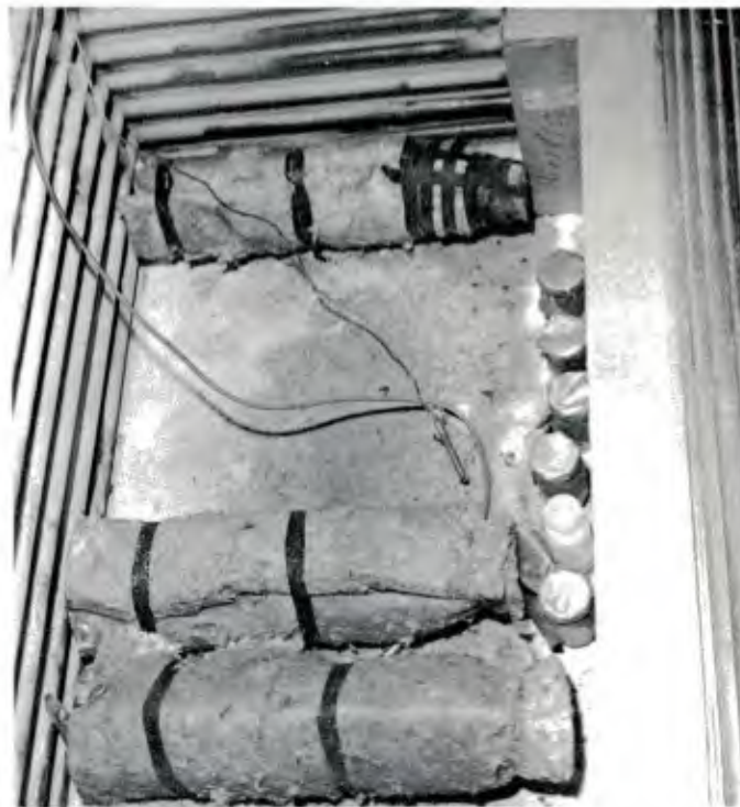
Figure 5. Extinguishers being cold-soaked.
