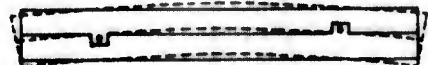
Figure 1-29. Element H, showing division of electrode plating for exciting fundamental mode. Similarly divided electrodes are on reverse side. The nodal "ears," where the mounting wires are attached, are at a distance of approximately 0.224 times the length from the ends*
