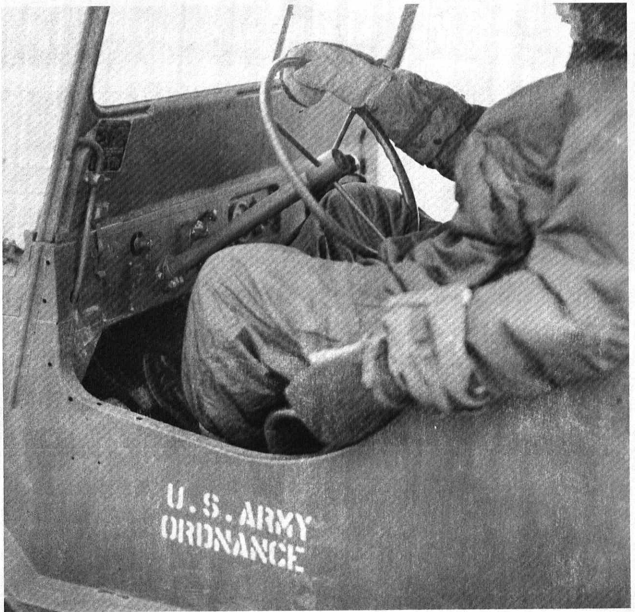
Figure 7. View Showing the Awkward Leg Movement Necessary to Operate the Brake.
