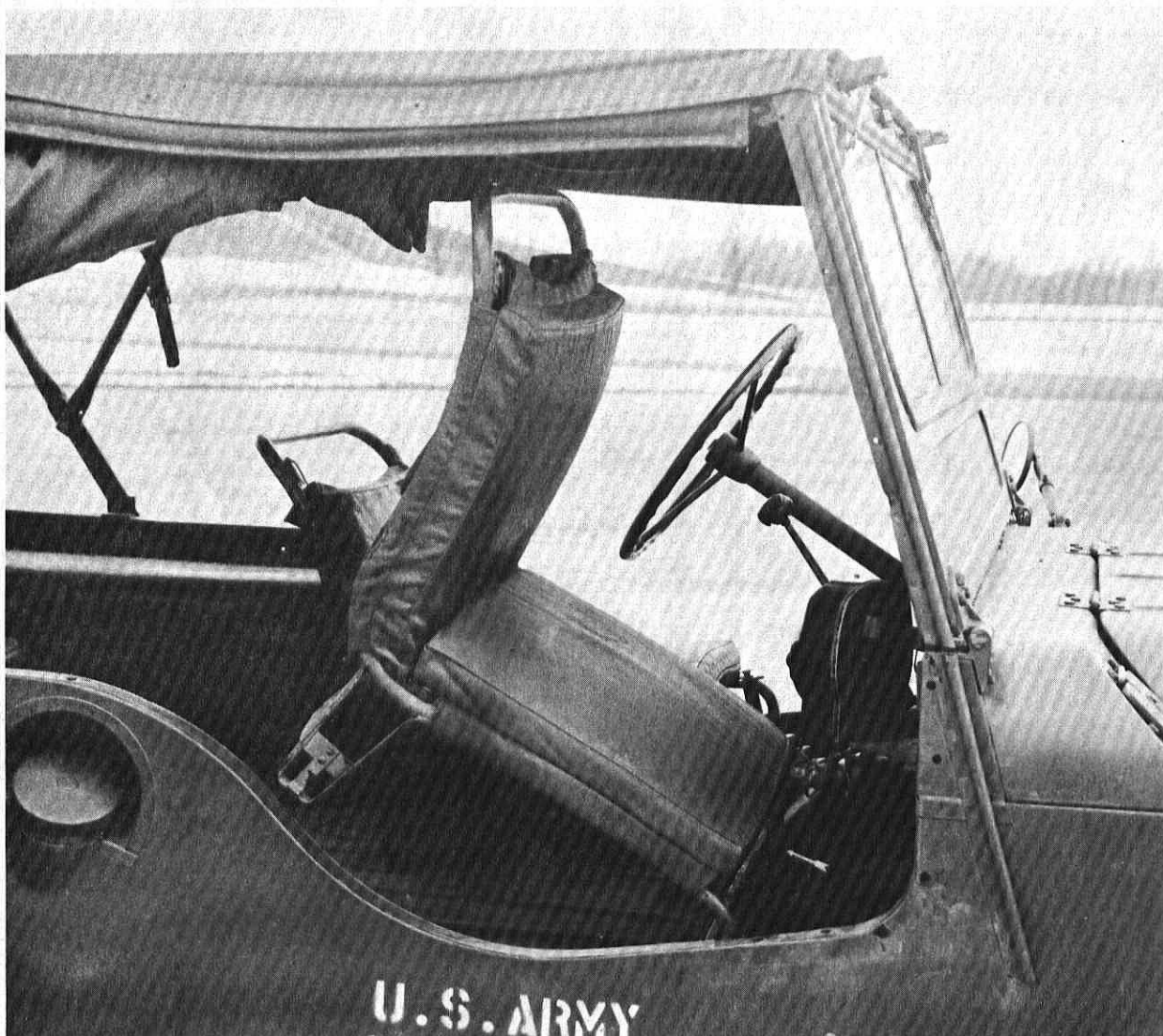
Figure 4. Inaccessibility to Rear Compartment due to Seat Leg Striking Shift Tower.
