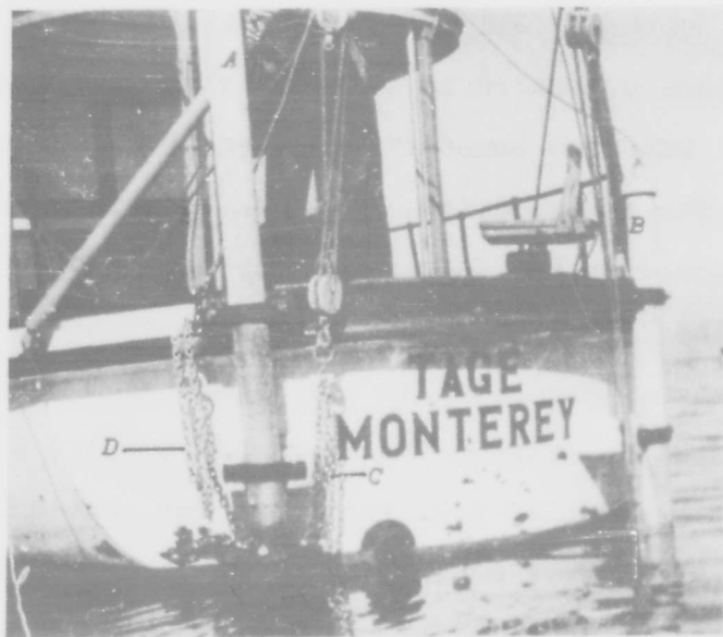
FIGURE 3. A VIEW OF THE STERN OF THE "TAGE" SHOWING THE SHALLOW RANGE TRANSDUCER (A) IN THE RAISED POSITION. BLOCK-AND-TACKLE SYSTEMS (C) ARE INBOARD. THE OUTBOARD CHAIN (D) SERVES AS A SAFETY STOP.
