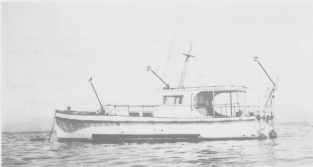
FIGURE 2. THE "TAGE" AT HER MOORING IN MONTEREY BAY. THE WINCH (A) CAN BE SEEN ON THE FOREDECK WITH THE TOWING WIRE RUNNING OVER A SHEAVE (B) MOUNTED ON THE PEAK OF THE CABIN AND OVER THE METER BLOCK (C) SUSPENDED FROM THE A-FRAME AT THE STERN.
