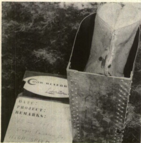
Figure 70 Blast Bag and Test Compartment
