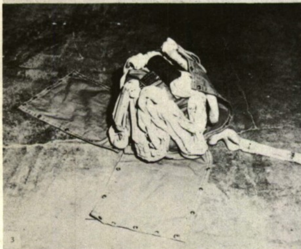
Figure 52 Cylindrical Bag-Packing Procedure and Closure Method
