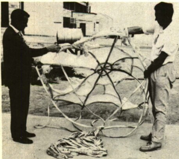
Figure 48 Damaged B7-8-20 (Modified) Rotafoil Parachute after Test Run No. 56
