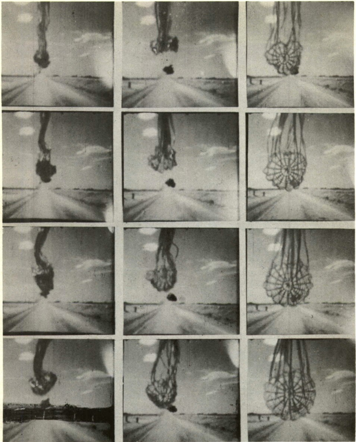
Figure 37 Inflation Sequence - FIST Ribbon Parachute Type 122 ( L_s/D_0 = 2 )
