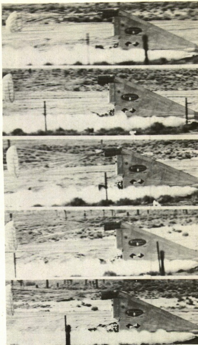
Figure 32 Deployment Sequence - FIST Ribbon Parachute Type 121
