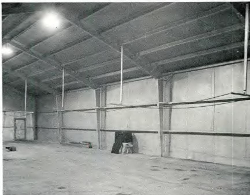
Figure 8. Cables suspended in shielded room for insertion loss tests.
