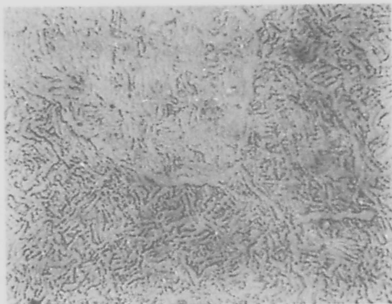
FIGURE 17. MICROSTRUCTURE OF VACUUM-ANNEALED Ti-2Cr-2Fe (K-26) SHOWING A MIXTURE OF APPROXIMATE 50 PER CENT ALPHA (WHITE) AND BETA (GRAY)
