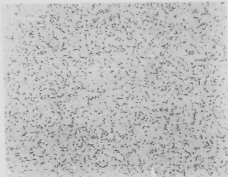
FIGURE 16. MICROSTRUCTURE OF VACUUM-ANNEALED Ti-6Al-4V (K-37) SHOWING SMALL PARTICLES OF BETA IN AN ALPHA MATRIX
