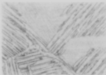
d. Coarse Acicular Alpha, Stabilized
