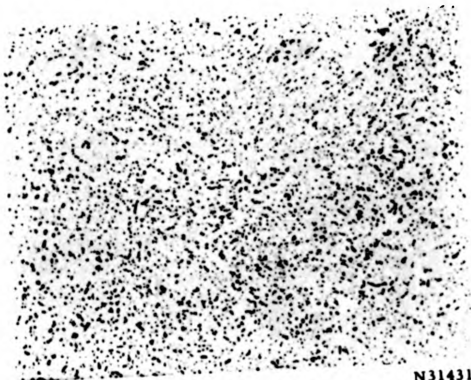
FIGURE 19. MICROSTRUCTURE OF VACUUM-ANNEALED Ti-4Cu (Ti-19) SHOWING PARTICLES OF COMPOUND (Ti 2 Cu) IN AN ALPHA MATRIX
