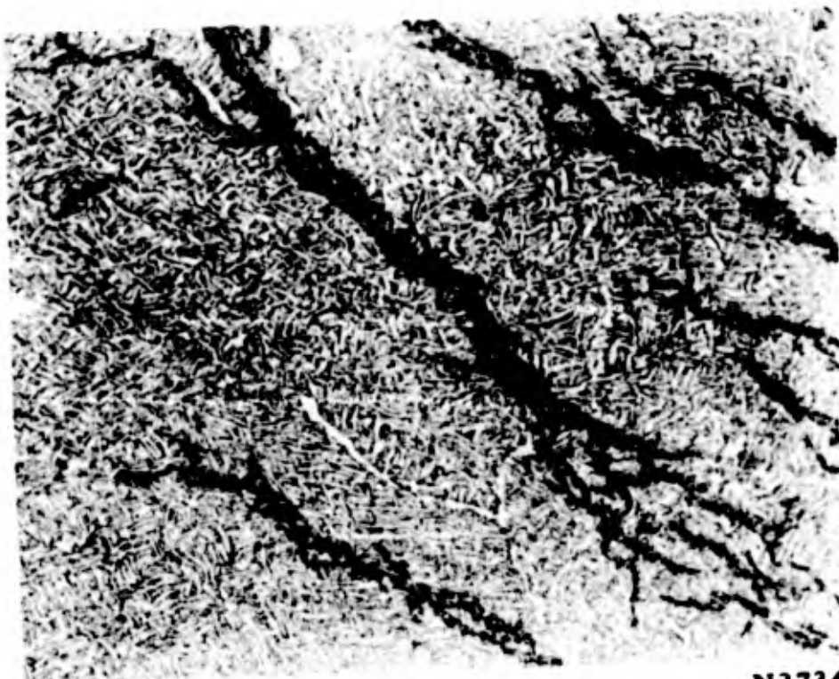
FIGURE 10. Ti-2Mo-2Fe-2Cr ALLOY CONTAINING 200 PPM HYDROGEN Solution heat treated and aged.
