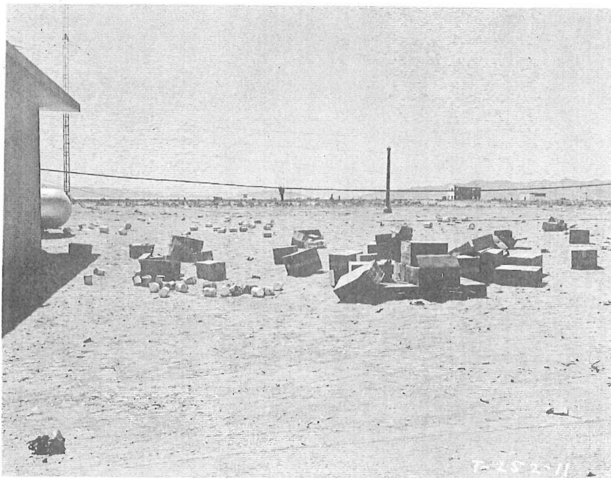
Fig. 4.23 — Pallet load scattered on the ground surface at 4700 ft from Ground Zero, following the blast.
