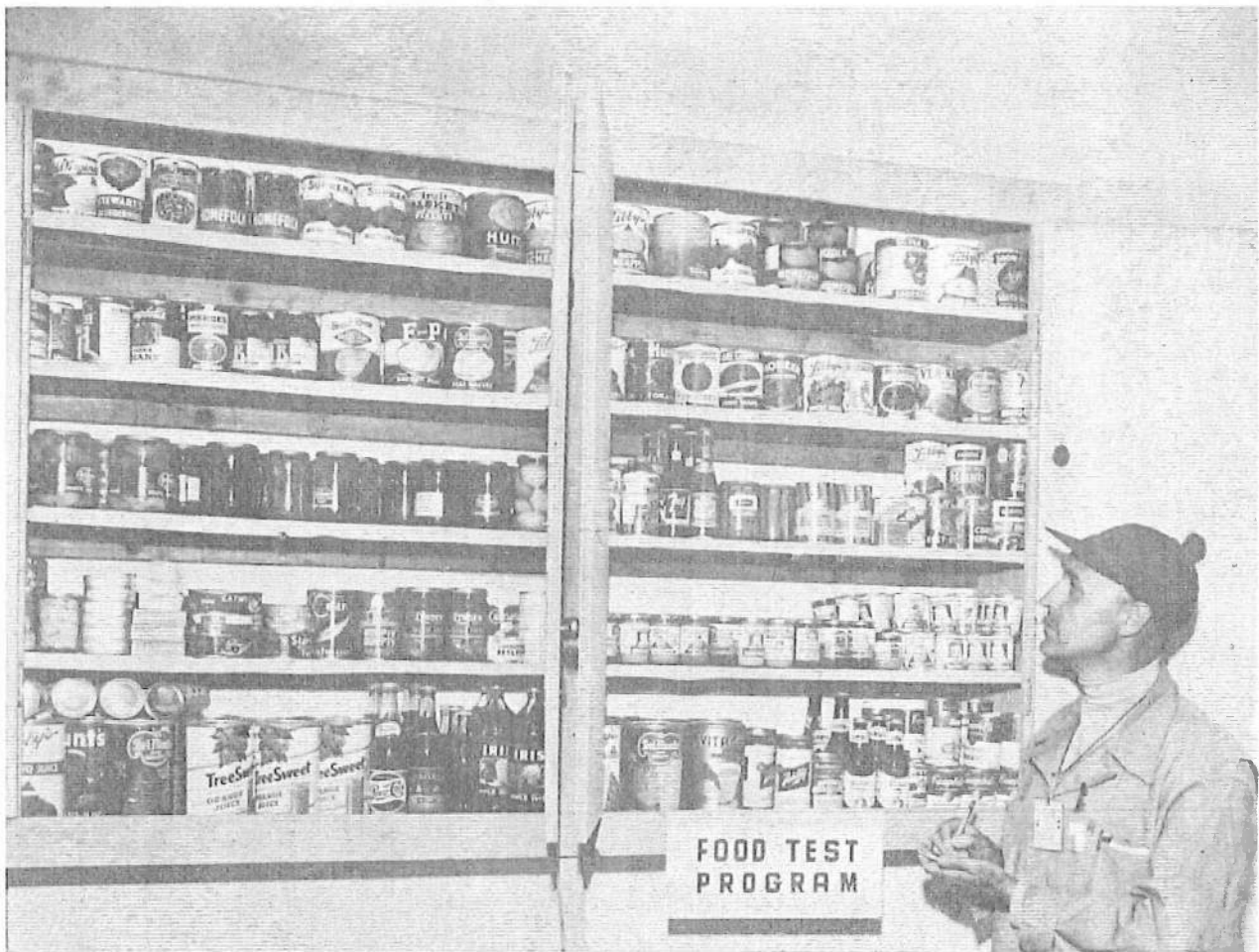
Fig. 4.13—Postshot view of kitchen shelves in precast concrete house at 4700 ft from Ground Zero.
