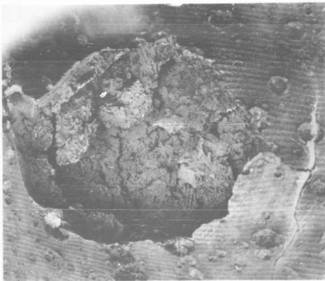
B25726: Rear view of 7-inch plate fired at 1000 yards, 60° obliquity - showing back spall of Round 10, depth of spall is 3/4 inch size of spall is 15" x 12". Interior of spall is laminated.
