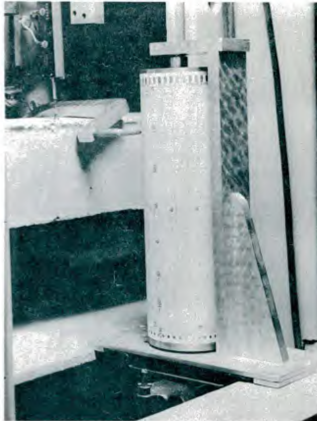
Figure 6. Rotating drum-deflection gage.
