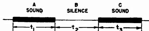
FIGURE 80. Sequence within a test pair, where time intervals t_1 , t_2 , and t_3 are equal.
