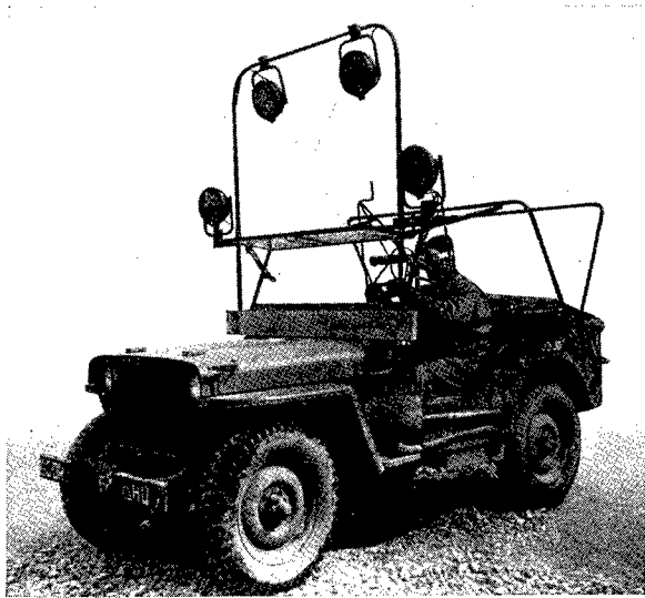
FIGURE 10. The equipment of Figure 9 mounted on \frac{1}{4} -ton truck. There are four 36-watt projectors; binocular image tubes mounted on springs in frame suspended from windshield frame and front bow. Binoculars are fastened to driver's head with web harness. The power source is a 12-volt battery strapped on the left sponson.
