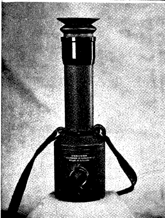
FIGURE 9. Type H metascope, front view and side view.
