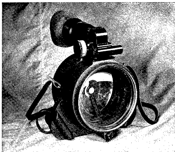
FIGURE 15A. Stadiometer for Type B, attached to metascoper.
