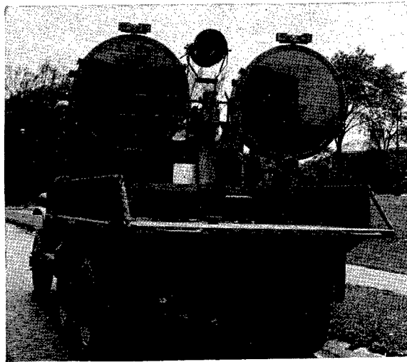
FIGURE 17. The 36-inch IR searchlights and 12-inch Schmidt receiver.
