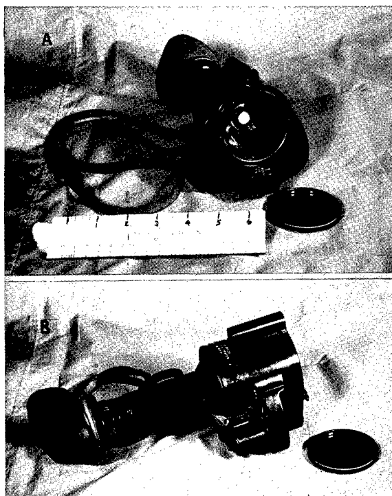
FIGURE 4. A. Front view of Type A metascope. B. Side view.
