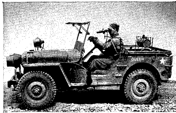
FIGURE 41. Jeep equipped for night driving with infrared.
