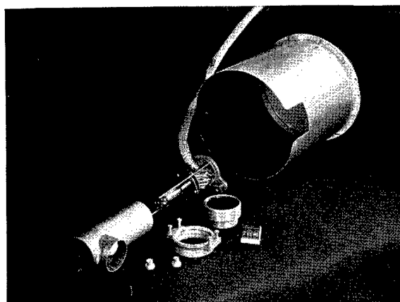
FIGURE 11. Photomultiplier receiver. Upper —Receiver assembled, mounted on tripod for field use. Seven-inch collecting mirror. Amplifier and power supply not shown. Lower —Receiver disassembled to show component parts.
