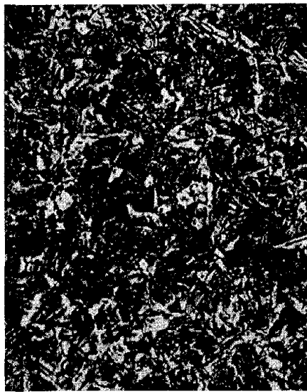
a. 1-inch section. Homogenized 1650°F - 300 min., air cooled; 1550°F - 90 min., water quenched. Tempered 1200°F - 30 minutes
