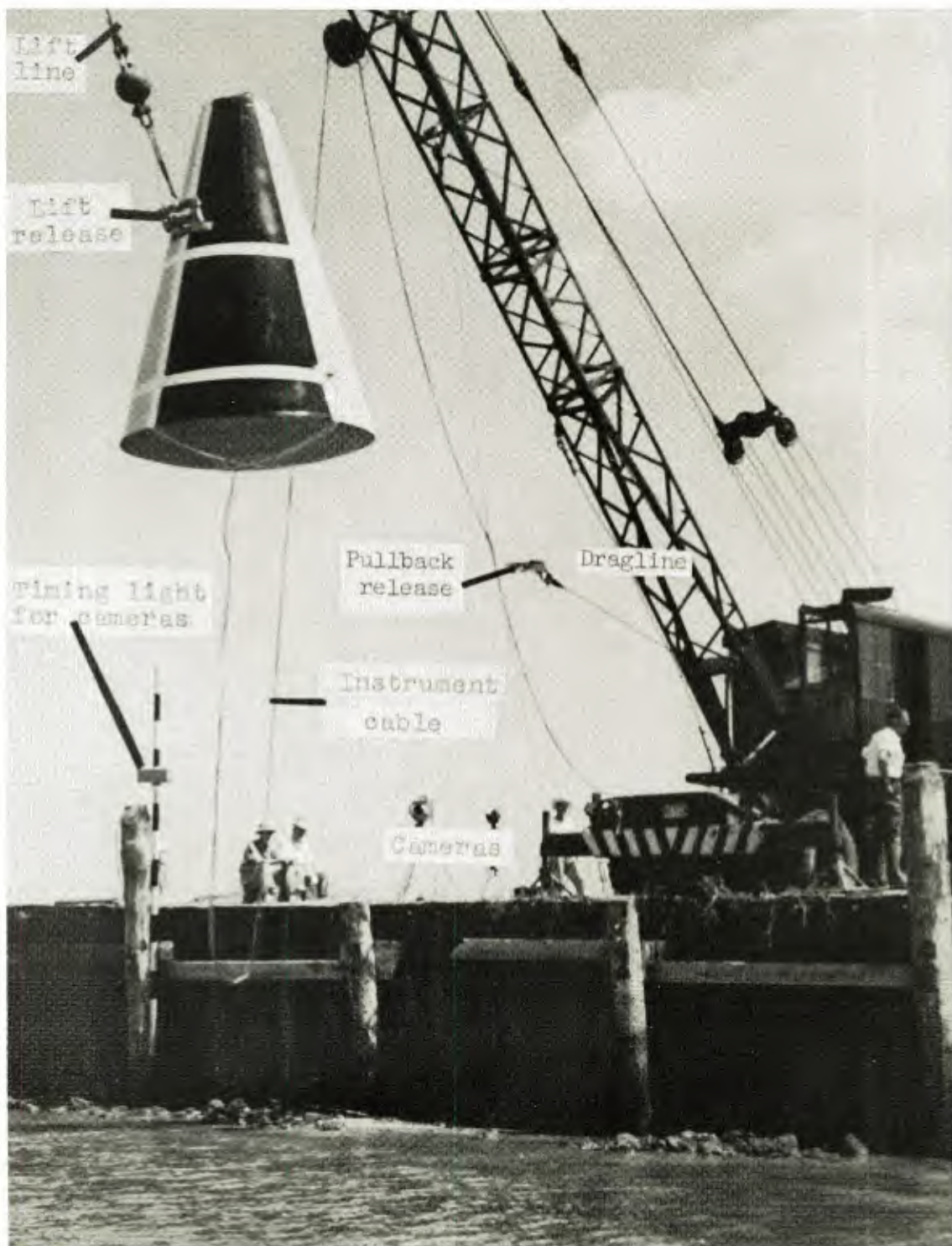
L-58-3338.1 Figure 4.- Full-scale test setup for nominal 65^{\circ} flight path and nominal 30^{\circ} attitude.
