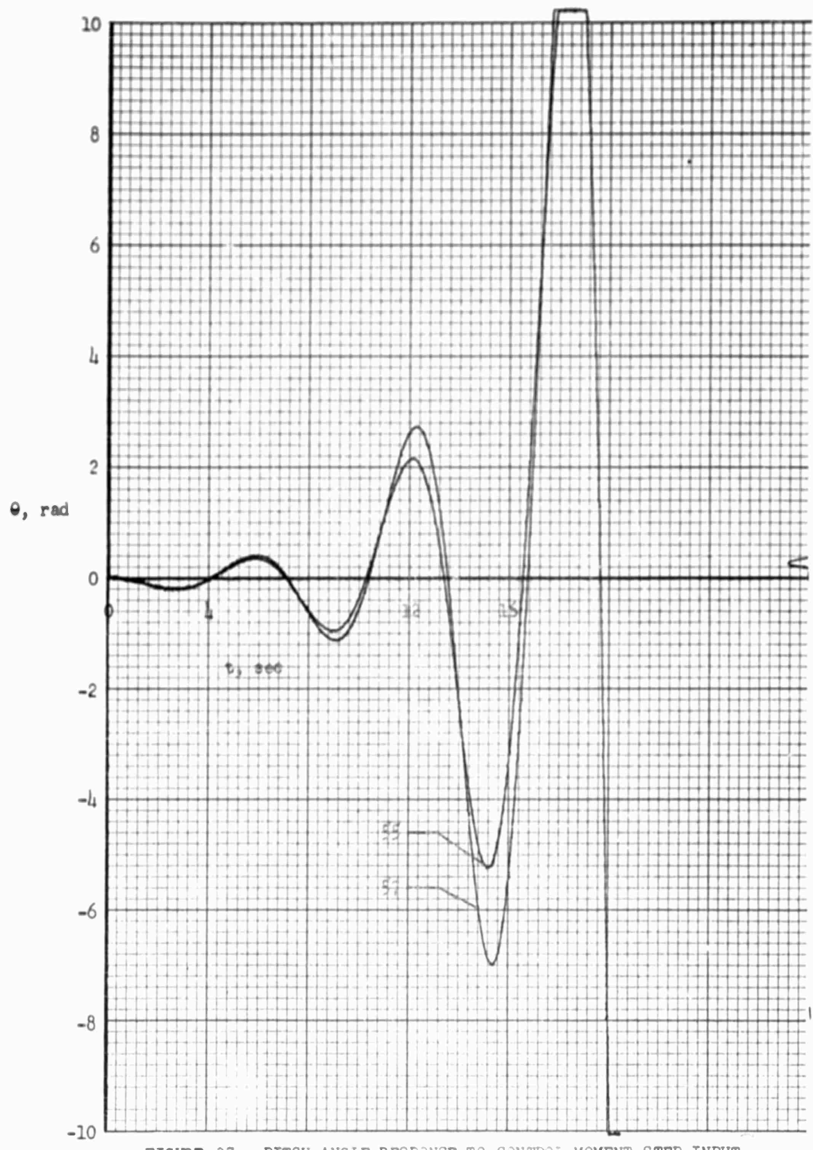
FIGURE 37: PITCH ANGLE RESPONSE TO CONTROL MOMENT STEP INPUT FOR CASE NOS. 55, 57
