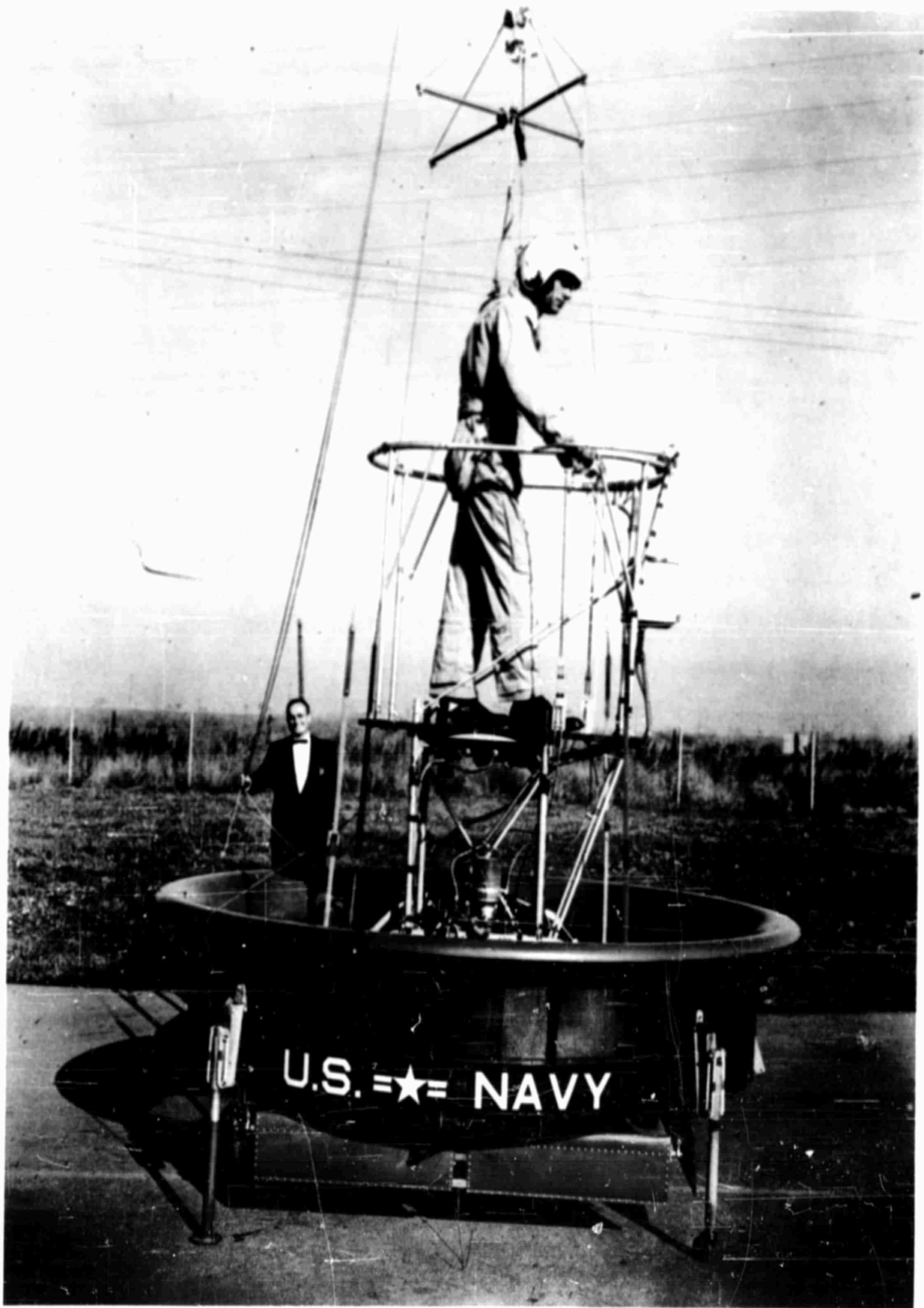
FIGURE 2: SEVEN FOOT PLATFORM WITH RAISED CG CONFIGURATION
