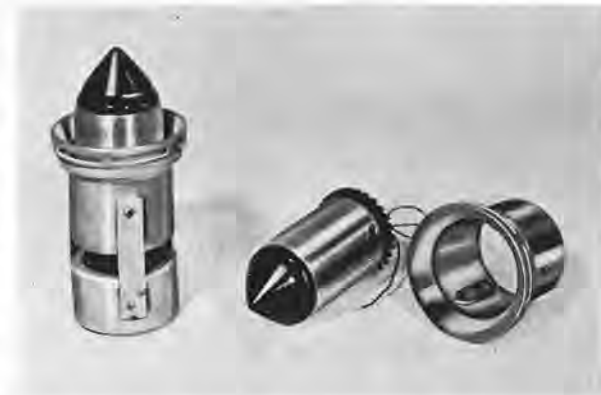
FIGURE 11. Photoelectric generator-powered rocket fuze, RPEG. At left, experimental model with improvised housing for arming switch SW-200 attached at rear. At center, electronic and power supply assembly. At right, cowl member for directing air to and from turbine.
