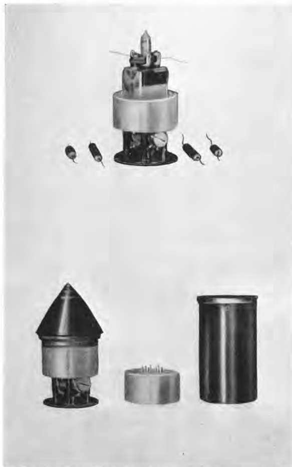
FIGURE 5. Views of RC time fuze for M-8 rocket. Top shows electronic components. Lower view shows, from left to right, assembled fuze with charging rings on ogive, switch, and fuze container. (University of Florida photograph.)
