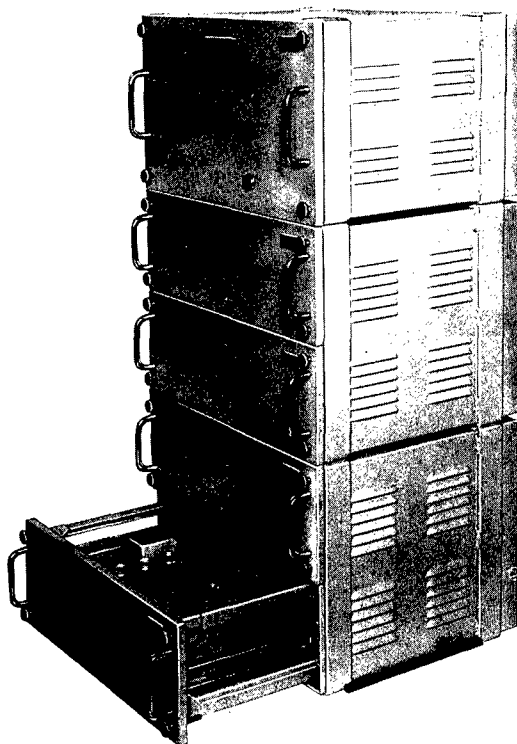
FIGURE 12. FM sonar Model 1, No. 5 (XQLA X-1) electronic stack (oblique view) (Submarine Spadefish installation).
