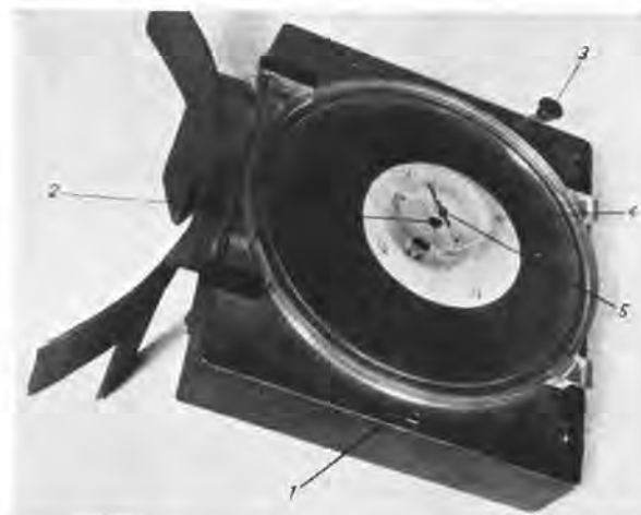
FIGURE 63. Top view of step-writer. (1) Thumb screw for orienting map paper, (2) knurled inking wheel, (3) plunger for distance input, (4) map paper, (5) compass needle.
