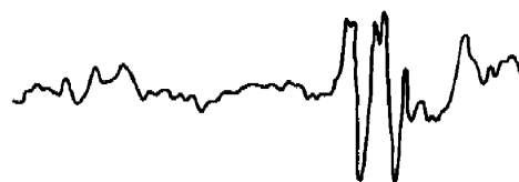
FIGURE 17. Oscillogram of single Canary motor. One cycle of a repeating wave. Fundamental frequency: 33 c; azimuth: 0 degree; distance: 1,000 ft.
