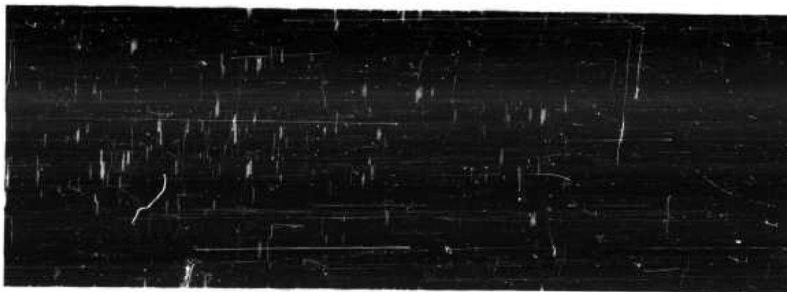
FIGURE 5. Appearance of copy scrambled by polarity reversal.
